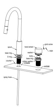
1.Drill a 35mm (for spout) and a 40mm (for mixer) through-hole on the counter. (The counter thickness must between 20mm to 40mm)
