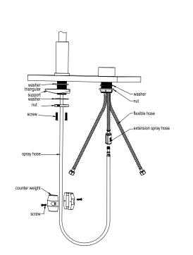
Slide rubber washer, triangle plate and steel washer and lock nut onto spout part in a row according above diagram. Then slide rubber washer and nut onto mixer part.
