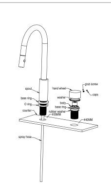
1.Drill a 35mm (for spout) and a 40mm (for mixer) through-hole on the counter. (The counter thickness must between 20mm to 40mm)
